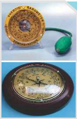
The offered barometer is widely used to teach the students the concept of How to measure air pressure and is greatly useful in laboratories.
