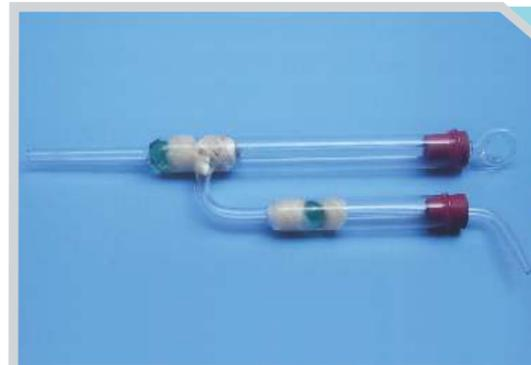
Demonstrates the working principle of the force pump, concept of double valve action of the pump and its ability to eject water at high pressure. Consist a glass cylinder with a non-return float valve at its lower end with an outlet side tube at its lower end, which in turn communicate the lower end of the secondary cylinder is equipped with a non-return float valve. The outlet tube from a secondary cylinder is drawn out into a jet.
