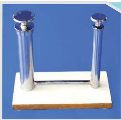
Demonstrates the process of transmissibility of fluid pressure. It consist of the plated cylindrical tubes of different diameters fitted with piston and connected to each other through a tube at their bottom. Piston have circular disc at the top for loading masses. Mounted on base.
