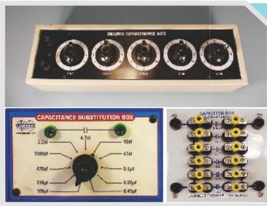
This decade Capacitance/Inductance substitution box provides 1, 2, 3 or 4 capacitors ranges from 100uF to 0.47uF with a resolution of 10%. The voltage range is 50volts AC or DC.
