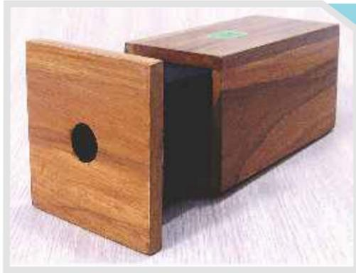
Two rectangular, open ended, light proof wood boxes. One slides into the other & contains a frosted translucent glass plate upon which image is formed. The other box has a pin hole opening at the closed end. Dimensions 150 x 100 x 100 mm approx.
