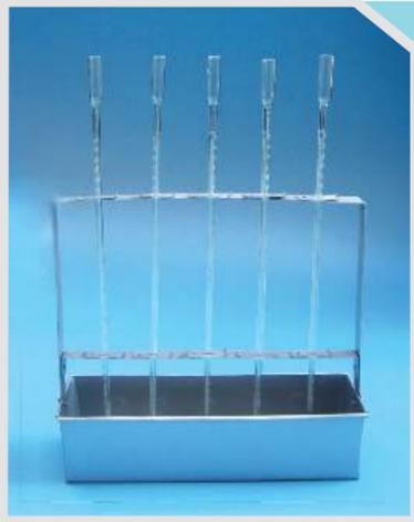
To show difference in expansion of various liquids over the same temperature range. It comprises 5 glass graduated capillary tubes of equal bore and bulbs at the bottom, mounted on a support frame with metal trough for immersion of bulbs in hot water in it.
